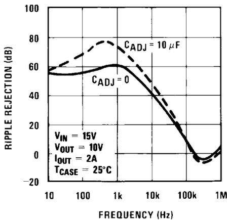
Figure 11. Ripple Rejection
