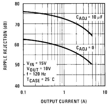
Figure 12. Ripple Rejection
