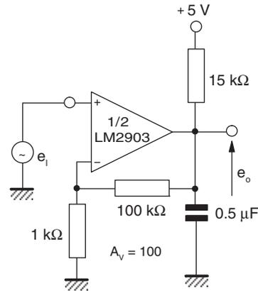
**Figure 12. Low frequency op-amp with boost**
