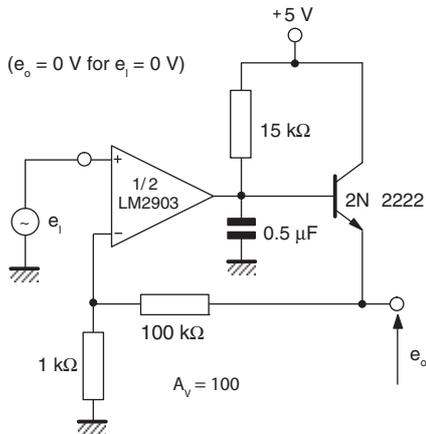
**Figure 13. Transducer amplifier**
