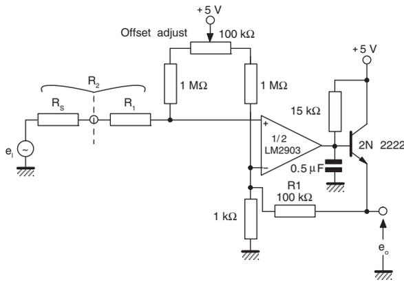
**Figure 15. Zero crossing detector (single power supply)**
