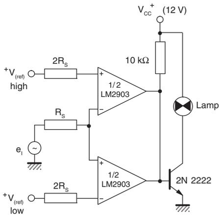
**Figure 17. Split-supply applications - zero crossing detector**
