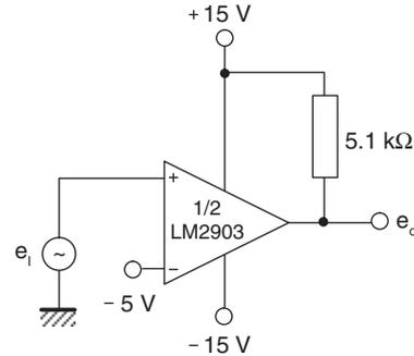
Figure 20. Time delay generator
