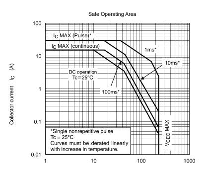
Collector-emitter voltage V<sub>CE</sub> (V)
